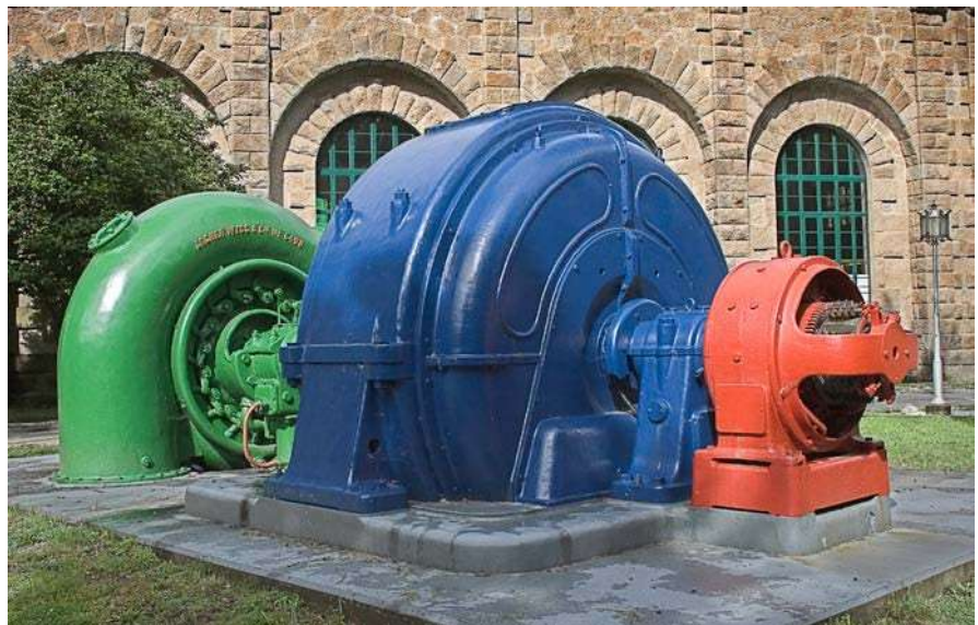
Image 91: Old turbine and hydraulic dynamo of the Tambre I power station.
